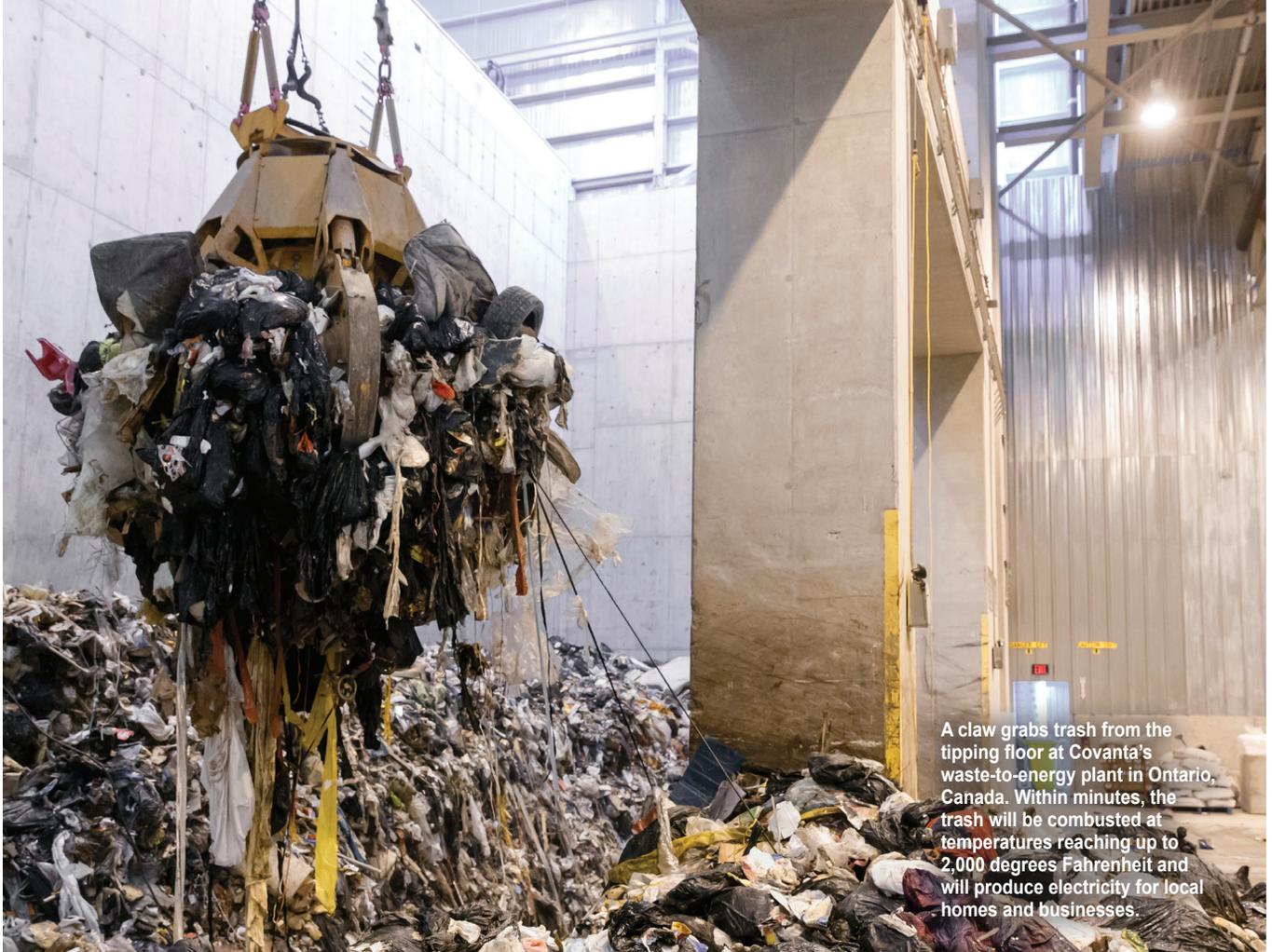
A claw grabs trash from the tipping floor at Covanta's waste-to-energy plant in Ontario, Canada. Within minutes, the trash will be combusted at temperatures reaching up to 2,000 degrees Fahrenheit and will produce electricity for local homes and businesses.
